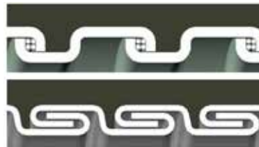
Square-Locked Design with cord packing 3/8" - 1-1/4"
